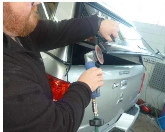
Grinding done on the corners
